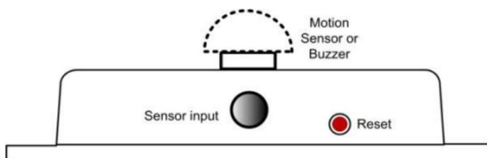
To reset the sensor to factory settings, press the button for about 5 seconds. Orange light will flash. Release button after the orange light is off. The sensor will restart into factory default mode.
